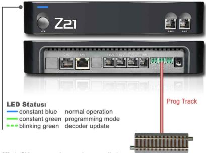
**Hint:** CV-programming can be cancelled by shortly pressing the STOP key.
